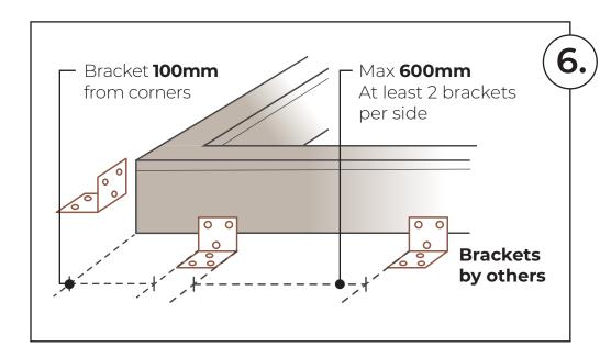
You can fix the upstand down with brackets. We recommend at least 2 brackets per side at **600mm** centres and **100mm** from each corner
